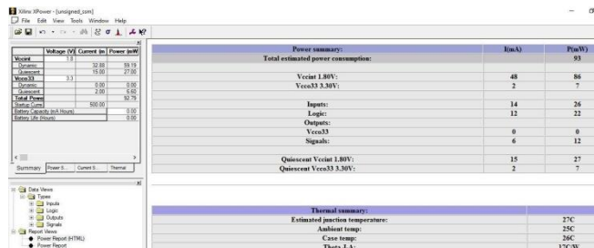
Figure 5.6: Power of dynamic segmented multiplier is 92 mW
