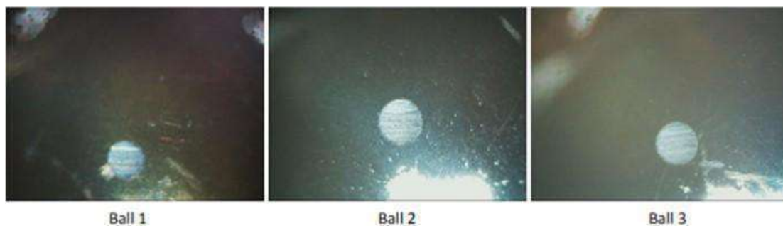
Fig 8 Wear scar for coated - test oil 3 sample
