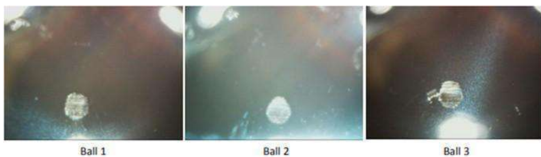
Fig 9 Wear scar for uncoated - test oil 2 sample
