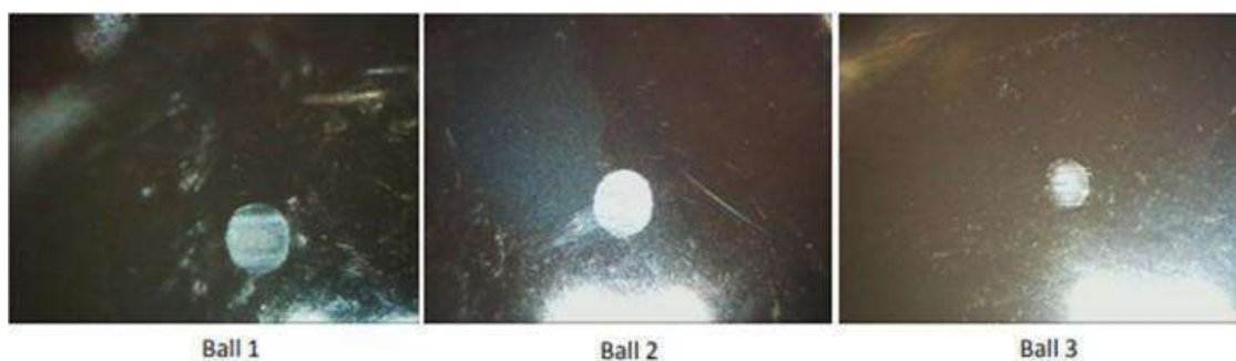
Fig 10 Wear scar for coated - test oil 2 sample
