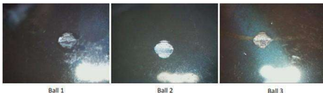
Fig 12 Wear scar for coated - test oil 1 sample
