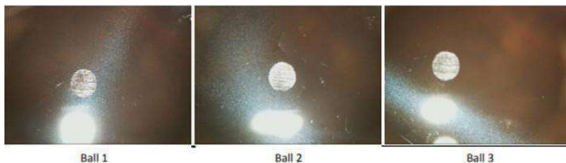
Fig 11 Wear scar for uncoated - test oil 1 sample
