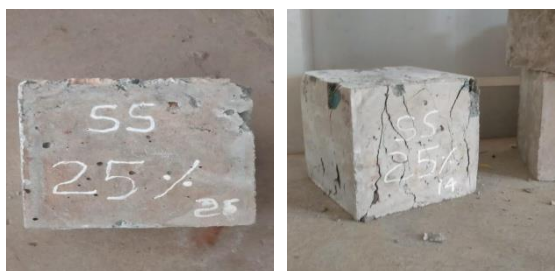
Replacement of Coarse Aggregate as Tile Wastes In Kg
