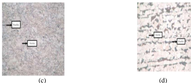
Fig. 3. Microstructure from S355J2G3 and S500M steel [22].
