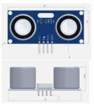
An ultrasonic sensor is an instrument that measures the distance to an object using ultrasonic sound waves. An ultrasonic sensor uses a transducer to send and receive ultrasonic pulses that relay back information about an object's proximity.
