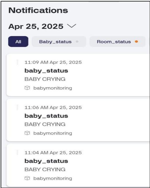
Fig 4 shows how the ESP32 delivers real-time notifications to parents through the Blynk IoT app, allowing remote monitoring and quick response to the needs of the infant.
