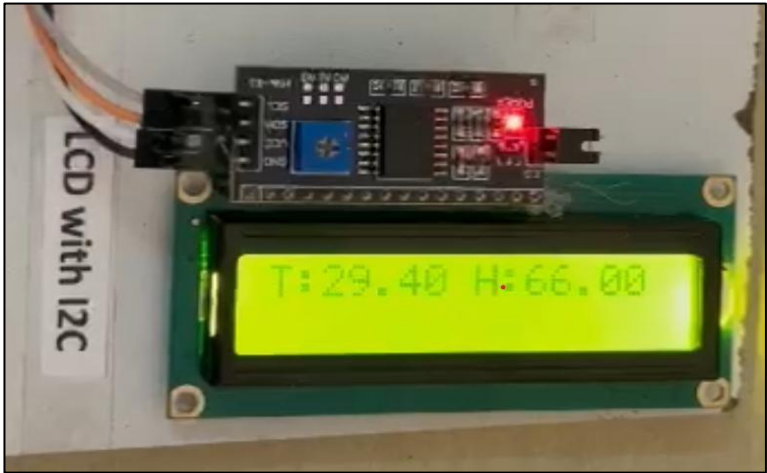
Fig 2 shows LCD with I2C displays real-time temperature and humidity data sensed by the system
