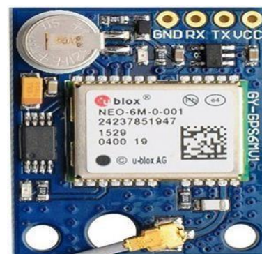
Fig.3.2 Pin Out of GPS Module
