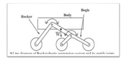
the suspension system has a "rocker" component. Through a differential, these rockers are linked to the chassis of the car as well as one another. To ensure roughly equal wheel contact, the rockers will rotate in opposite directions with respect to the chassis. The average pitch angle of both rockers is maintained by the chassis.
