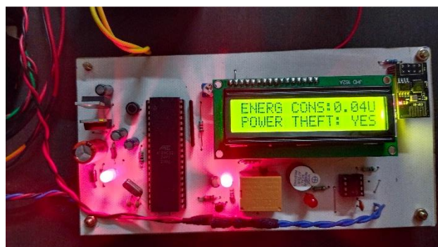
Fig3: LCD Display when power theft
