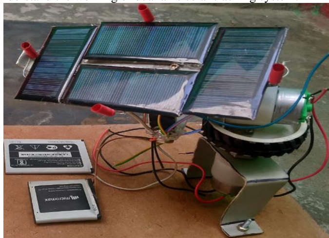
Fig. 3 Proposed model of dual axis solar tracking system
