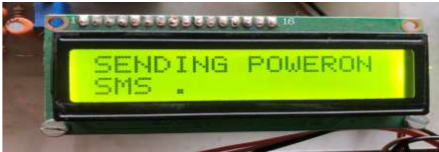
Fig. 1- Once the switch is turned on, the system sends activation message.
