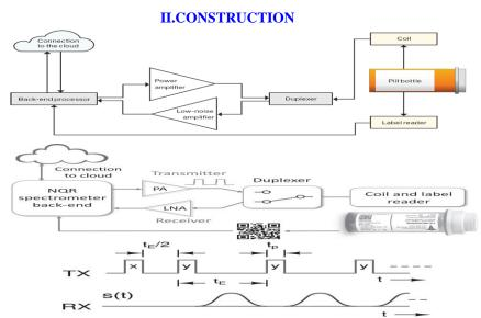
It consists of cloud connection, back to end NQR spectrometer, transmitter, receiver, duplexer and coil and label reader. Prototype NQR equipment includes six fundamental blocks, including one designed for reading the label on a pill bottle. The back end controls the excitation pulses and converts the amplified output of the coil sensor to digital form for further analysis, which is performed elsewhere through a connection to the Internet.
