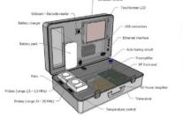
Prototype portable screening device for packaged medicines Mounted in a rugged carry case Dimensions: 33cm x 53cm x 19cm Weight: ~ 8 kg Battery or mains powered
