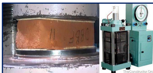
Figure 5: Compressive Strength Test on Brick using Compression Testing Machine
