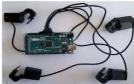
Figure 3. Arduino Mega based board and current sensors.
