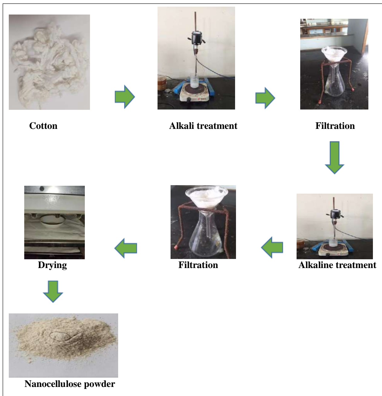
Figure 2. Flow diagram of isolation of nanocellulose from cotton
