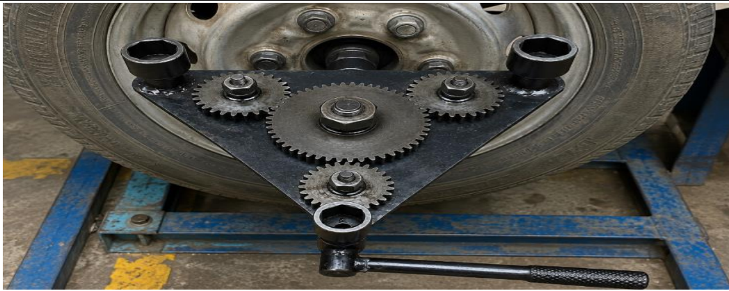
Figure 5. Experimental Testing Setup of Multi Nut Tightened Mechanism
