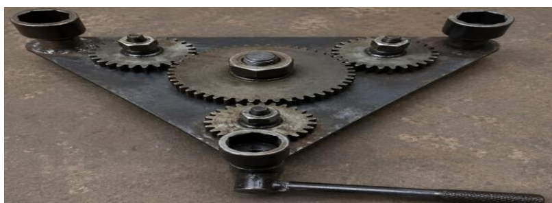
Figure 2. Real Fabricated Model of Manually Multi Nut tightened and Loose Mechanism.
