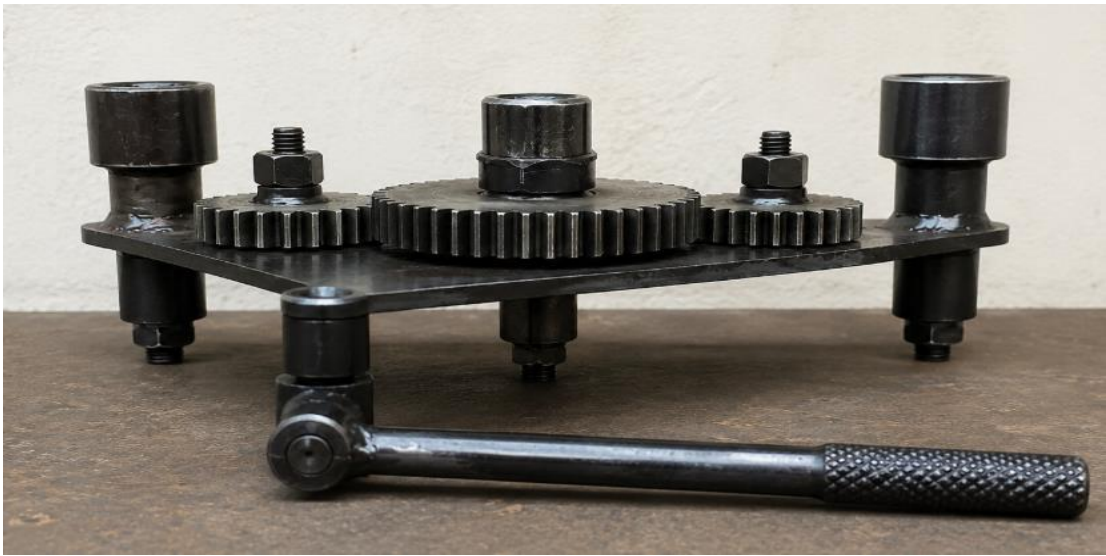
Figure 4. Side View of Fabricated Multi Nut tightened Mechanism
