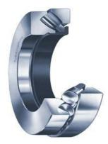
Tapered roller bearings are designed to support large radial and large thrust loads. These loads can take the form of constant loads or shock loads. Tapered roller bearings are used in many car hubs, where they are usually mounted in pairs facing opposite directions. This gives them the ability to take thrust loads in both directions. The cutaway taper roller on the left shows thespecially designed tapered rollers and demonstrates their angular mounting which gives their dual load ability.
