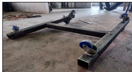
Figure (4): Wheels welded on the base
