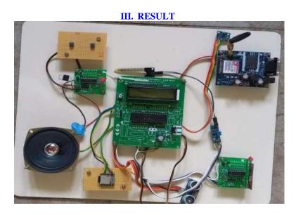
The Lora TX/RX gives the message about the bus arrival and the location of they needed place as audio message. When the blind person stuck at emergency the GSM module send the signal to their guardian. The result is shown as screenshot.
