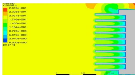
Figure 17: Fin Spacing of 6.5 mm
