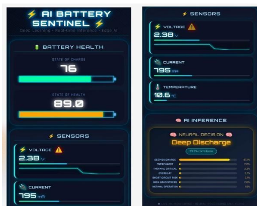
Figure 7. AI Battery Sentinel dashboard showing real-time battery health, sensor readings, and intelligent battery-state classification under deep-discharge condition.
