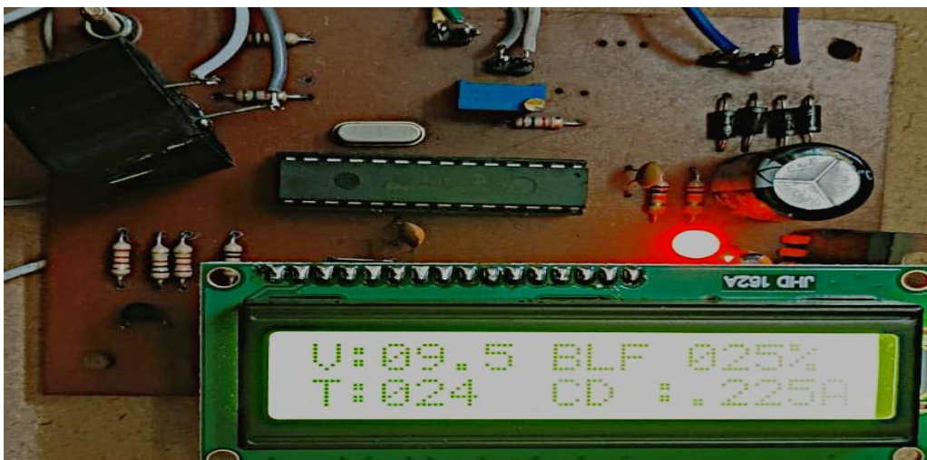
Figure 3: shows the results of Iot based battery management system
