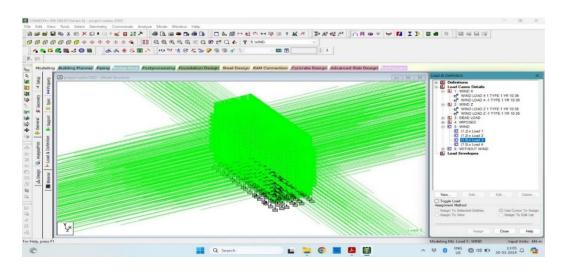
Dead Load: 9 KN/M, Live Load: 18 Kn/M Wind Load: 2 KN/M At The Top Of The Building
