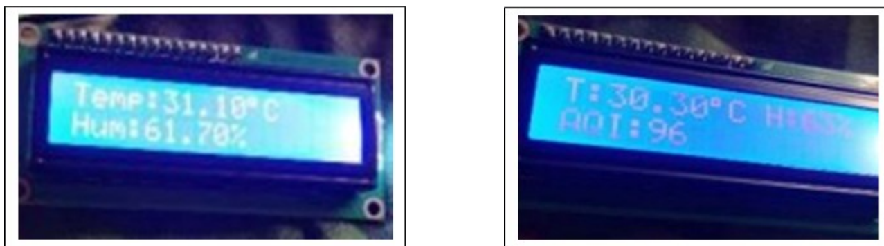
Fig. 6. Prototype LCD output showing real-time environmental parameters
