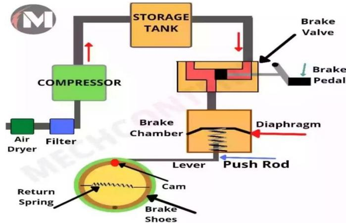
2) **AIR FILTER**- Air Filter is used Before the Compressor to remove the Dust Particals from the Air, before entering in to the Compressor.
